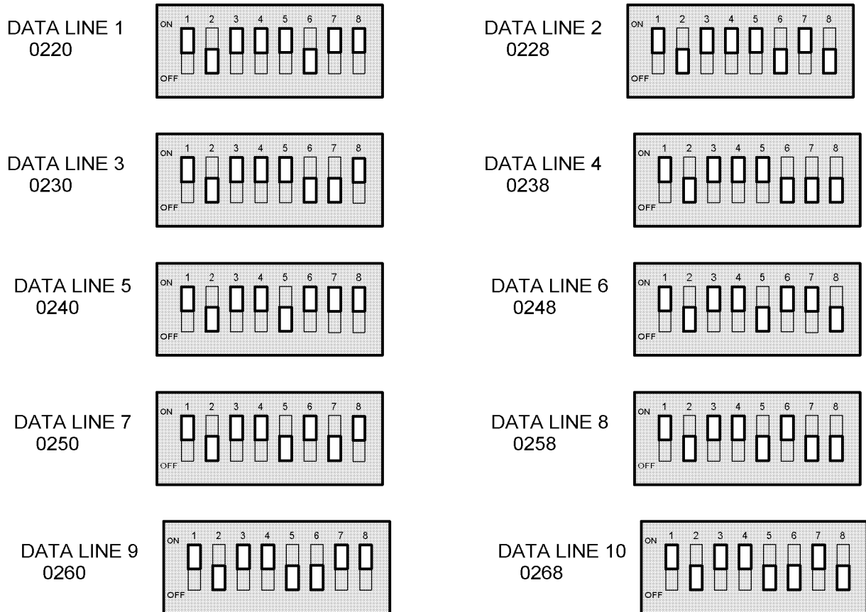
Figure 3 Typical HM-501 Serial Interface switch settings
